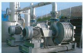
Two (2) Model 077.06 blower packages with Control Panels and VFDs for OEM installation in Germany.
